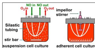
Figure 4 – Membrane Diffusion Delivery System for Nitric Oxide
